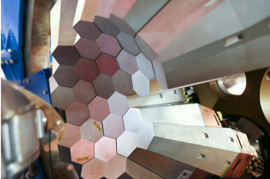
FIGURE 1.4: AGATA sub-array with 32 crystals arranged in 10-triple clusters and 1-double cluster installed at GANIL in France.
