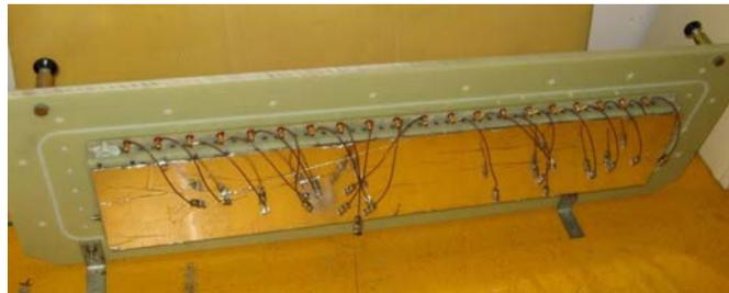
FIGURE 2.12: Picture of the MWPPAC assembly taken from Ref. [45].
