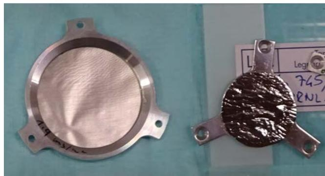
FIGURE 2.18: Picture of the  $^{92}\text{Mo}$  target (right) and  $^{24}\text{Mg}$  degrader (left) used in the experiment.
