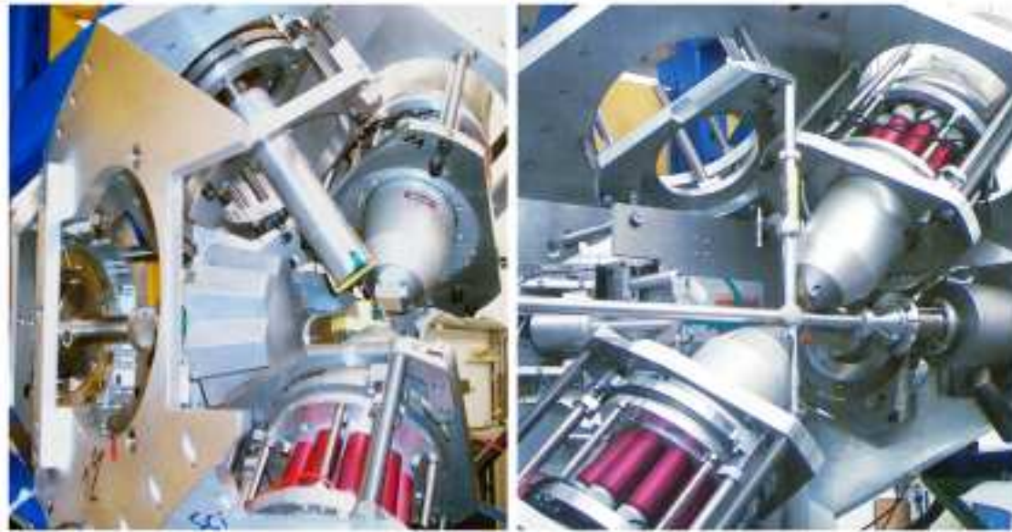
Figure 2.2: Picture of the detection system mounted in the Würfel frame designed at the IKP institute. The Würfel frame was opened in order to visualize the detectors. In the left picture, the CLUSTER detector which is beside the other Ge detectors can be seen, while in the right picture, we show the rest of the detectors and the beam tube.
