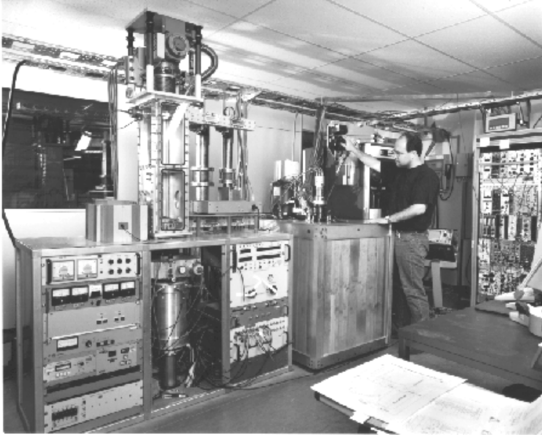
Figure 2.6: Picture of the TAS setup. Left: the implantation chamber above the last quadrupole of the beamline. Centre: outer part of the TAS shielding. Right: (large) experimenter and the station used for the tape transport behind him.
